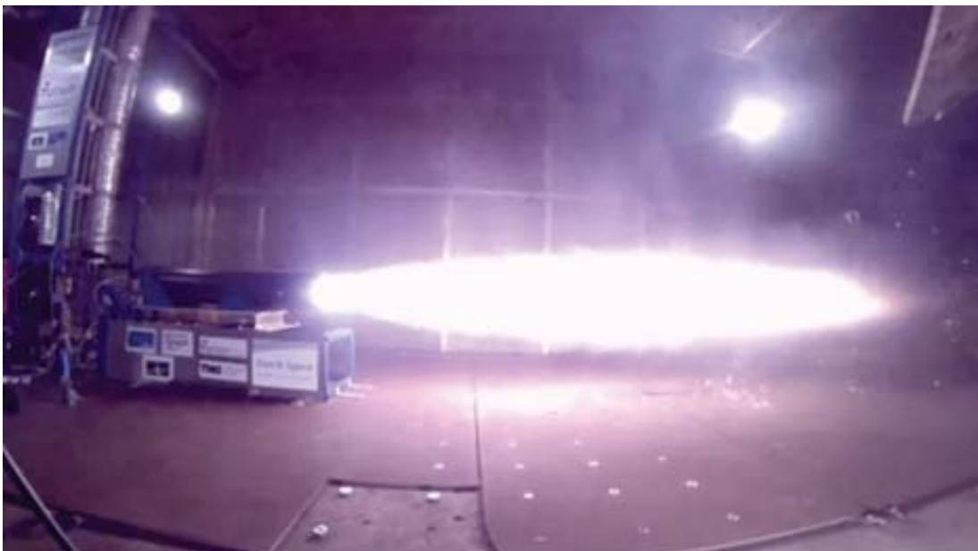
Figure 1.3: Still from the video footage of the hybrid rocket engine test at TNO in May 2013.
